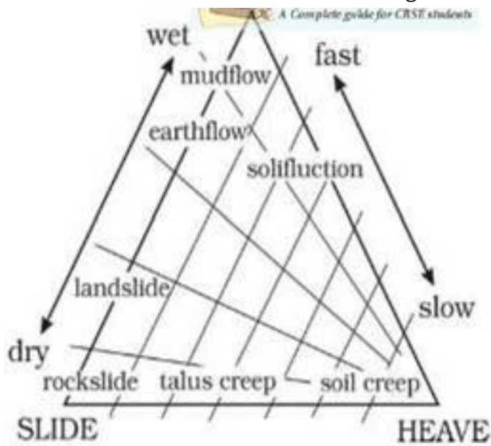
Figure 6.5 : Relationships among different types of mass movements, their relative rates of movement and moisture limits (after Whitehead, 2001)
